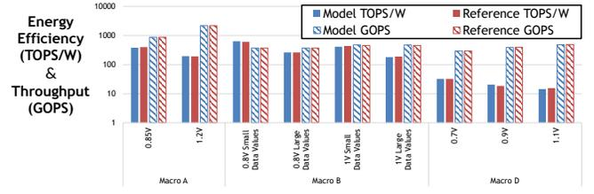
Fig. 7: Validating energy/throughput for varied supply voltage.
