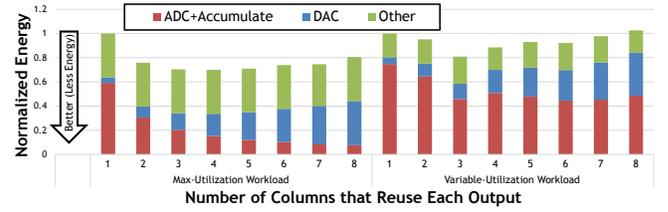
Fig. 12: **Macro A + Mapping:** Output reuse between columns decreases ADC energy but trades off lower input reuse and higher DAC energy. The three-column-reuse case had the best-utilization mappings for the variable-utilization workload.
