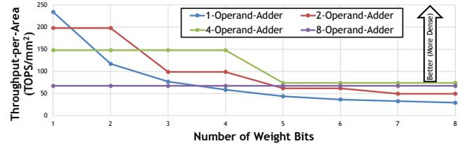
Fig. 13: **Macro B + Circuits:** An analog adder trades off flexibility for compute density. Fewer-column adders can flexibly leverage fewer-bit weights, but more-column adders achieve higher compute density with more-bit weights.
