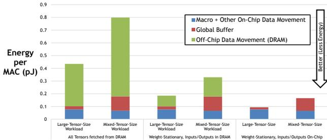
Fig. 15: **Macro D + Full-System**: Weight-stationary CiM saves significant energy, but benefits are limited by off-chip movement of DNN inputs/outputs between each layer. CiM will be most effective when combined with layer fusion to keep all tensors on-chip.
