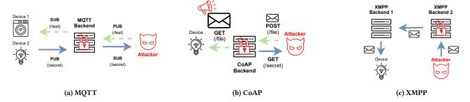
Figure 1: Attack Vectors for the Studied IoT Protocols. We consider three different architectures: Publish-Subscribe (MQTT), Client-Backend (CoAP), and Distributed Client-Backend (XMPP). The colored arrows signify different flows.
