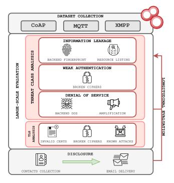
**Figure 2: Methodology Overview.** We first collect our backends' dataset via Shodan. Then, we perform our large-scale evaluation for the identified threat classes. For TCP-based protocols (i.e., MQTT and XMPP), we also evaluate TLS adoption and implementation. We repeat our analysis over time to understand how security posture evolves, and to consider the impact of our coordinated disclosure.
