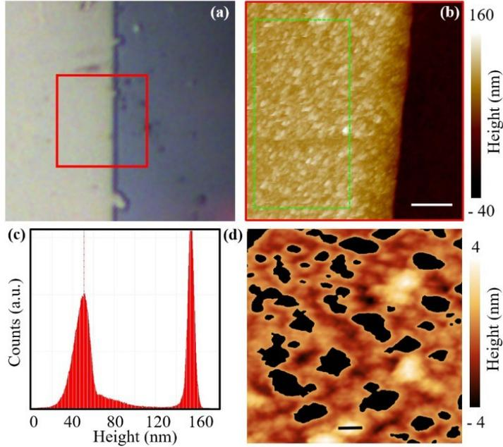
**Figure S3.** (a) Optical image of the Au/Si substrate. (b) AFM image of Au/Si substrate showing a thickness of the Au film to be  $\sim 100$  nm. (c) Measured size distribution of the region highlighted by a dashed green square in (b), confirming two size distributions centered at 50 nm and 150 nm respectively. (d) Dark mask AFM analysis confirming the presence of the two sizes ( $\sim 50$  nm and  $\sim 150$  nm) of Au grains.
