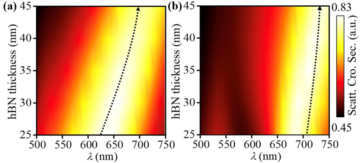
**Figure S8.** Color density plot of hBN layer thickness dependent spectral evolution of scattering cross section for the proposed system (a) without and (b) with 98-nm SNC.
