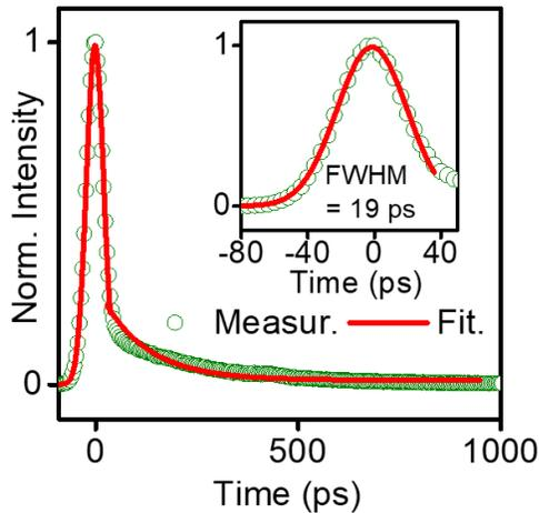
**Figure S4.** Instrument response function of the lifetime resolved optical setup. The solid lines are (a) nonlinear and (b) linear fits of the measured IRF, leading to a resolution for our setup equal to 21 ps.
