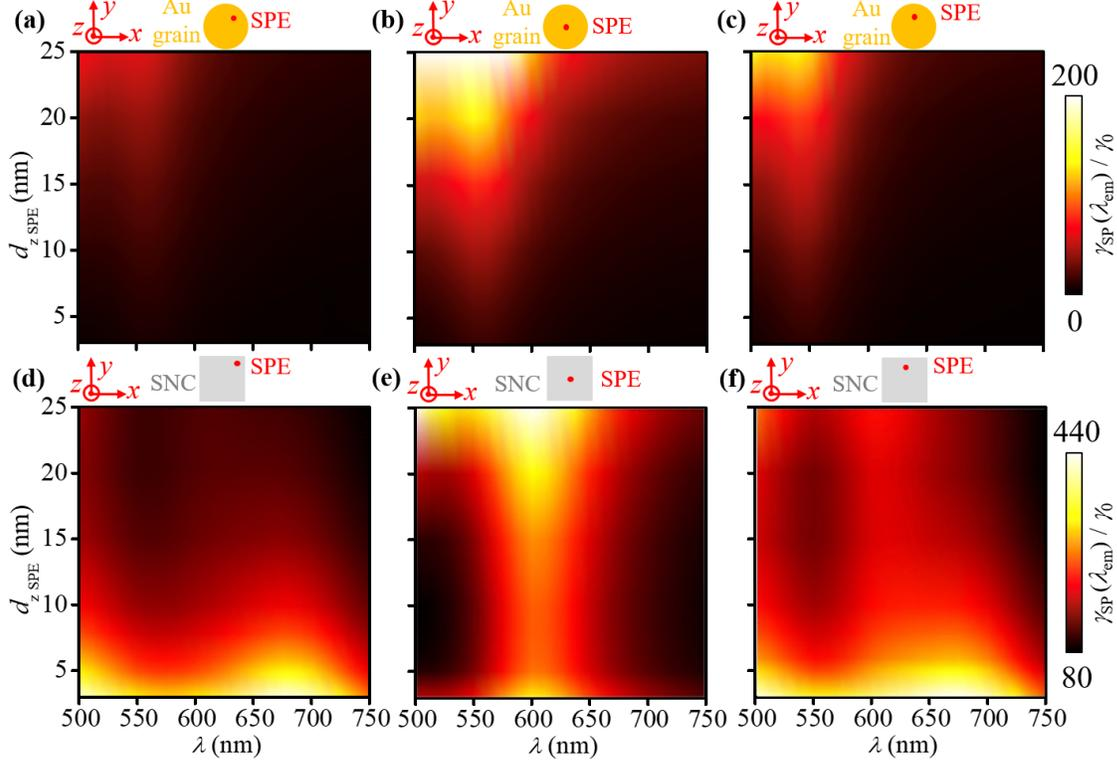
**Figure S9.** Color density plot of hBN layer thickness dependent spectral evolution of the normalized spontaneous emission rate ( $\gamma_{sp}/\gamma_0$ ) for the nanostructure without (a, b, and c) and with (d, e, and f) SNC for different emitter locations which are schematically illustrated on top of each figure.
